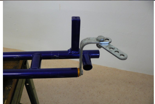
Photo from above of the frame with the section of the two supports for the exhaust system
